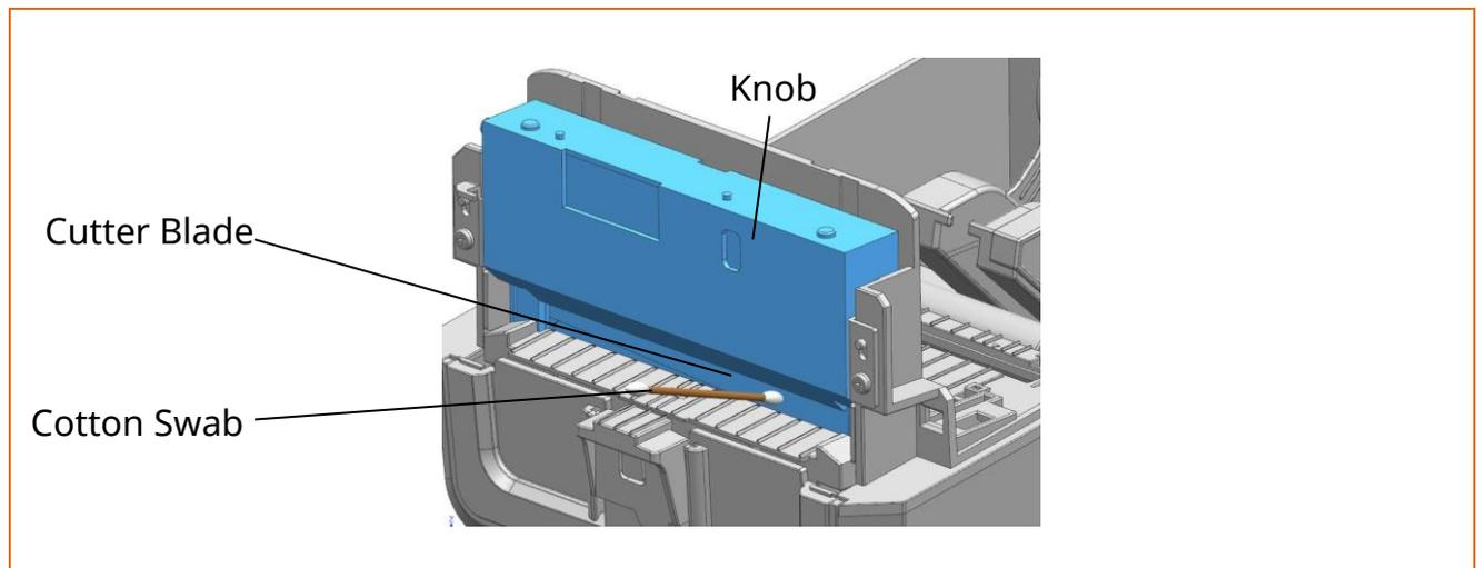
4) After the cleaning is complete, wait 1~2 minutes the alcohol of printer to evaporate completely, then reassemble the auto cutter cover in reverse process.
