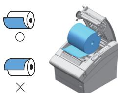
1. Push the Cover Open Button to open the Printer Cover.
