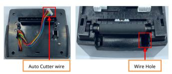
6. Insert the Auto Cutter Wire into the Auto Cutter Connector (red square) in the correct direction.
