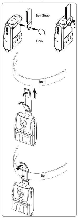
1) Insert the belt strap screw into the belt strap hole.
