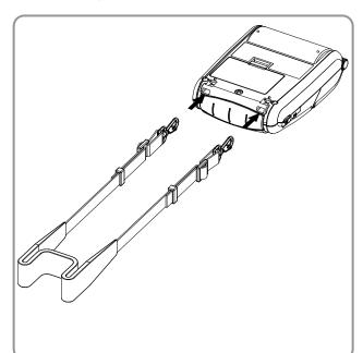
1) Connect the clips of the shoulder strap to the printer as shown in the figure on the left.
