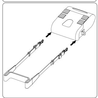
2) Connect the clips of the leather case as shown in the figure on the left.
